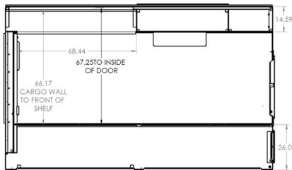
With this top down view, you can see the floor space available to install equipment and see how your portable equipment will fit into the space.
